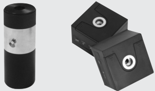
Calibrators for microphones and sound level meters. Reproduction of sound pressure level 94 dB and 114 dB at 1000 Hz frequency. Calibration accuracy 0,3 dB.
